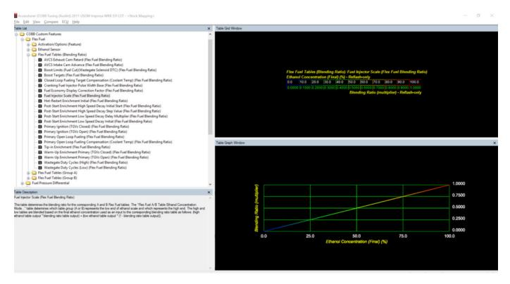
Ex: Fuel-Based Tables: linear blending from E0-E100 for Fuel Injector Scale
