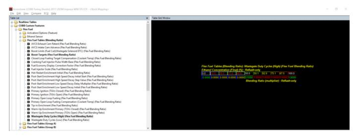
Ex: Octane-Based Blending Ratio table to introduce binary WGDC duty cycle control. Below E50, Group A tables are used, above E50, Group B tables are used. A minor blend will occur if ethanol content equals exactly 50.0%. Using a sensor deadband of greater than 1.0% will help eliminate this possibility, as raw measured ethanol content must change more than 1.0% before Ethanol Content Final is updated.
